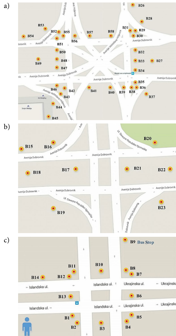
Figure 7. Network of beacon devices: a – starting point of movement; b – possibility of transport mode change; c – complex traffic intersection in the vicinity of various areas of interest
