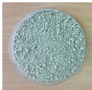
Figure 2. Zeolite granules (source: compiled by author)
