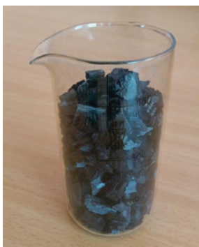
Figure 4. Biochar cubes (source: compiled by author)
