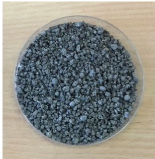
Figure 3. Granulated foam-glass (source: compiled by author)
