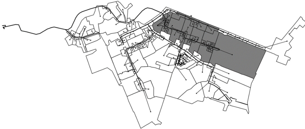
Figure 2. Scheme of existing stormwater drainage system and rainwater catchments connected to junctions
